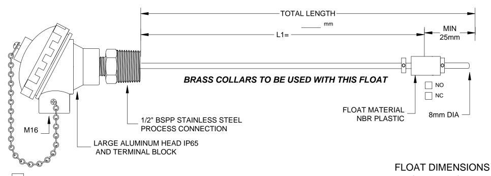
STANDARD - NO or NC CONTACT RATED AT 32V AC/DC @ 500mA RESISTIVE LOAD
